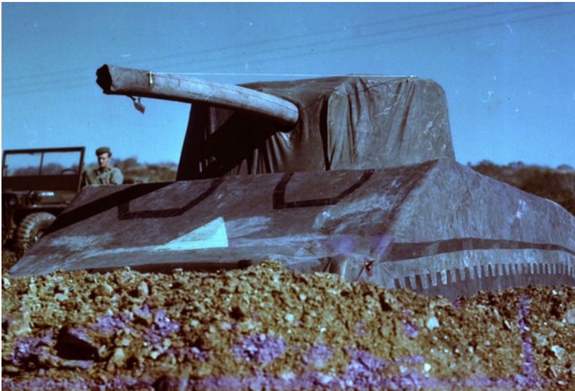
A 93-pound inflatable tank, of the kind used by the Ghost Army (National Archives)
